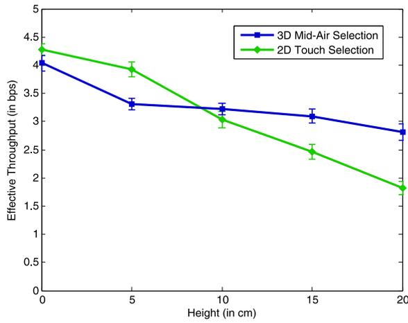
**Figure 6: Effective throughput metric combining errors and movement time: The horizontal axis shows the target height, and the vertical axis shows the movement time. Higher throughput is better. The error bars show the standard error.**
