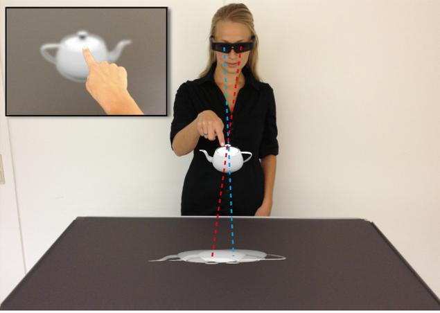
**Figure 2: Illustration of the main problem of 3D mid-air interaction with stereoscopically displayed 3D data: The user sees a stereoscopic image while converging to her finger, but due to the vergence-accommodation conflict, the virtual object appears blurred in comparison to the finger.**
