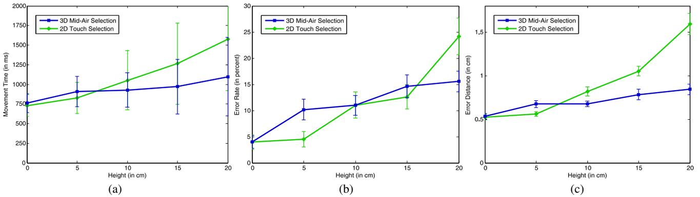
**Figure 5: Results for Fitts' Law trials with target object height on the horizontal axis and pooled for (a) movement time, (b) error rate, and (c) error distance, on the vertical axis. The error bars show the standard error.**
