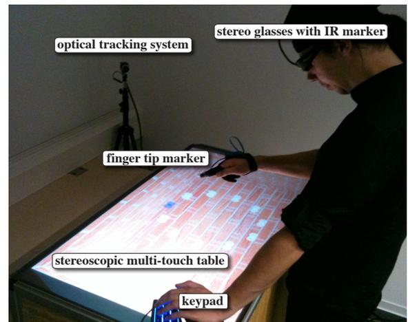
Figure 4: Experimental setup: photo of a subject during the experiment with illustrations.
