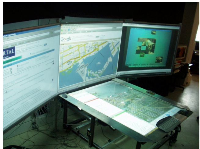
Figure 4. An overview of the screen configuration of MULTI. All projectors and cameras are located behind the screens. The image on the table is created by two projectors (partially located underneath the middle wall screen).
