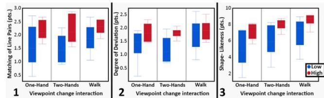
Figure 9: Experiment 2 results, 1) matching of line pairs, 2) degree of deviation, and 3) shape likeness.
