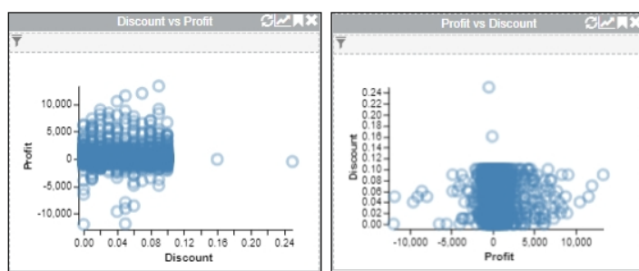
Fig. 4. The axes of a chart are swapped using the transpose option. The transpose icon is left-most in the icon bar at the top-right.
