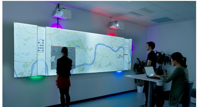
Figure 1: Using ambient light to support work on large interactive surfaces via peripheral information display.
