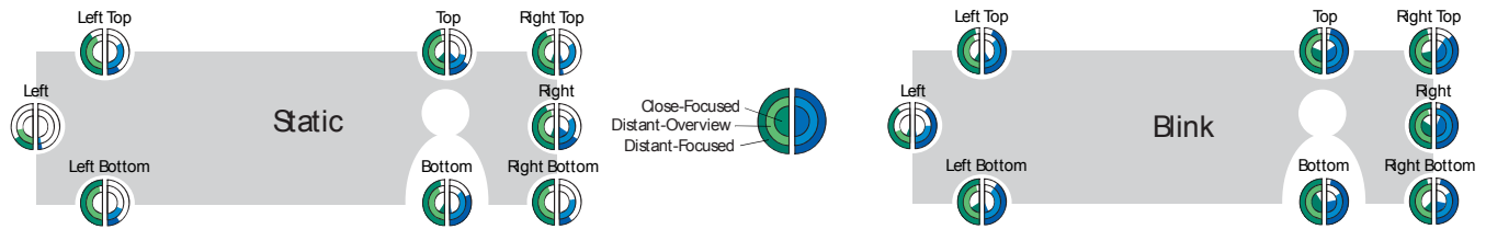
Figure 5: Perception of notifications in different spots. The green part of the circles shows the recognition rates for Ambient Light, the blue part the rates for on-screen notifications.
