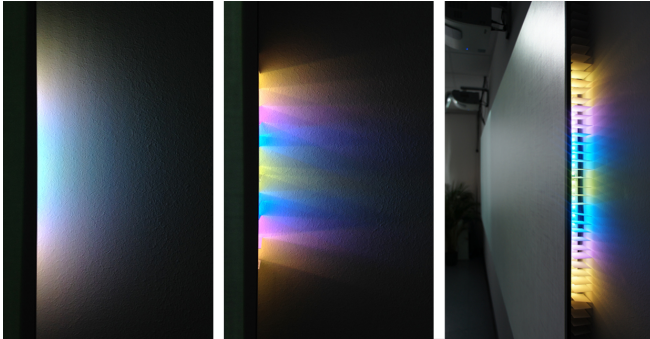
Figure 10: Comparison between ambient light with and without separators. Left: The light blends and different colors can hardly be distinguished. Middle: The separators prevent the blending of colors to make identification easier. Right: The separators in the whiteboard context.
