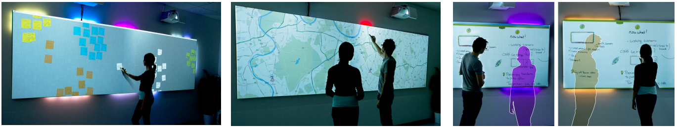
Figure 12: Example applications. Left: Off-Screen content visualization in a virtual 2D workspace; Middle: Visualizing notifications; Right: Indicating the position of a remote user – the colored silhouettes are not part of the actual visualization.
