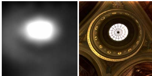
Figure 11: Factorization of an HDR photograph for the LED-based display. Left: LED contribution as a result of convolving LED values with the LED point spread function. Right: edge enhanced LCD panel image that corrects for the blurriness of the LED image.
