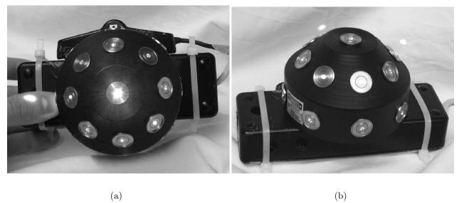
Figure 5: The Hedgehog hardware. 17 laser diodes are arranged in a symmetrical hemispherical arrangement. As shown in (a) the IS-900 tracker is rigidly attached for experimental purposes.
