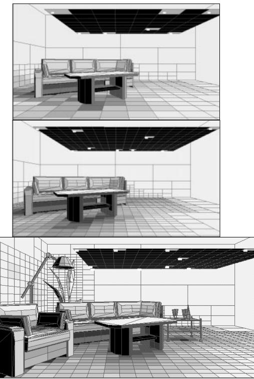
Figure 4: Visualization of solutions for simple environment (top and middle) and for complex environment (bottom). The global viewing region is the large dark polygon near the ceiling, viewing regions are shown in medium gray and small white rectangles depict viewpoints. The color of each surface element encodes how many viewing regions can see it.
