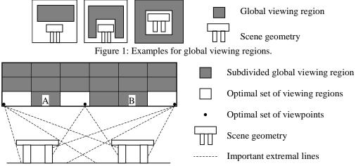
Figure 2: Scene with two tables, a global viewing region, and an optimal set of viewing regions and viewpoints (see text).
