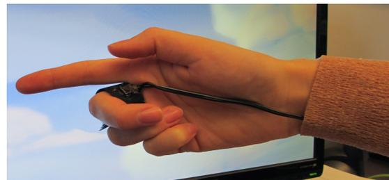
Figure 6: Photo of finger ring with the button visible below the users thumb (raised more than normal for illustration). Self adhesive tape was used to keep the cable from interfering with the motions.
