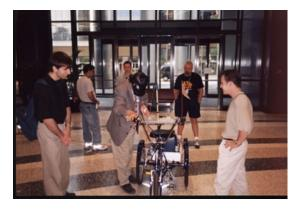
Figure 1: The Virtual Reality Tricycle. The VR Trike permits different combinations of visual and non-visual cues to be presented to an operator, but uses a HMD to generate the visual cues.
