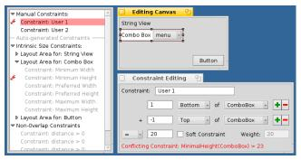
Figure 14. Left: Constraint list. Top-right: Editing canvas. Bottomright: Constraint edit dialog. The selected constraint "User 1"  $(ComboBox_{height} = 20)$  conflicts with the minimum height constraint of the combo box  $(ComboBox_{height} \ge 23)$ . Conflicting constraints are marked in the list and the corresponding widget is highlighted.
