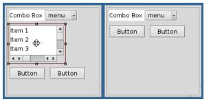
Figure 11. Filling gaps: Upon removal of the list widget, the two buttons both "float" vertically. Moving the button group up fills the gap. The tops of the buttons are connected to the bottom of the combo box.
