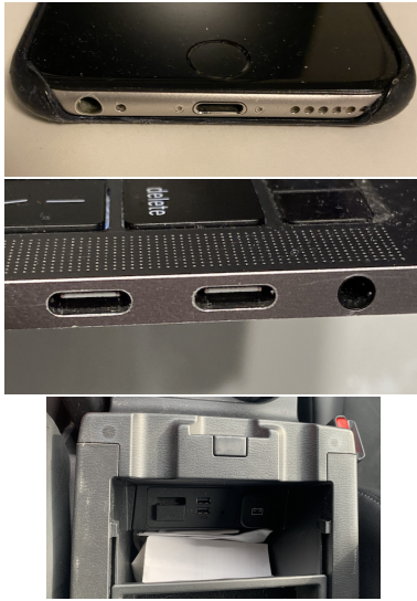
Figure 2: Left and middle: Example for devices where there are multiple different receptacles clustered together in a constrained space. Right: Ports in the center console of a vehicle photographed in late afternoon on a sunny day. Note that even though there is a lot of light, the ports are not that easily visible.
