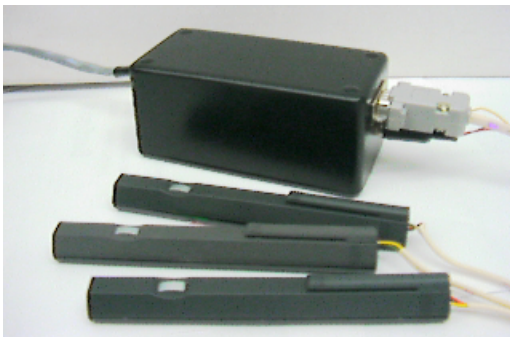
Fig. 6. Three computer controlled laser pointers and the box containing the electronics to control them.
