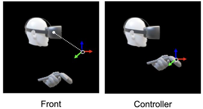
Fig. 3: The FRONT scaling center is located at a fixed position relative to the user’s head, set at a fixed offset at initialization. The CONTROLLER scaling center coincides with the dominant hand controller or the midpoint between controllers for bi-manual interaction.
