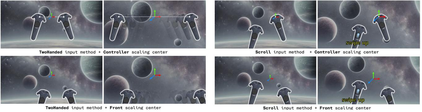
Fig. 4: The four variations of scaling techniques for exocentric navigation in multiscale virtual environments, resulting from the combination of two input methods for scale control (TWO-HANDED, SCROLL) and two methods to specify the scaling center (CONTROLLER, FRONT).
