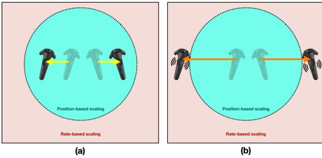
Fig. 7: Position-based scaling was used when the arms were within the inner region (blue) and rate-based scaling when outside (reddish). In the experiment, the inner and outer regions were not visualized to avoid a visual distraction. Instead, the two controllers vibrated (only) when they were in the outside region.
