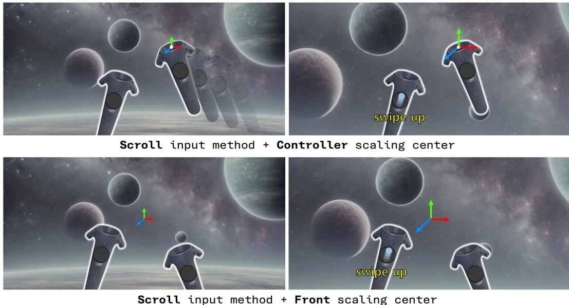
Fig. 1: Two novel scaling techniques for exocentric navigation in multiscale virtual environments, each using a different method to specify the scaling center (CONTROLLER, FRONT), all evaluated in our user study in comparison with the state-of-the-art two-handed pinch/grab-based technique (TWO-HANDED).
