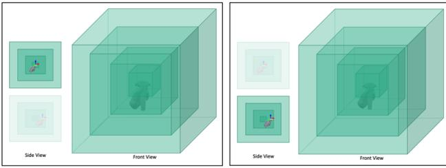
Fig. 2: A depth ambiguity occurs when an object, a controller in our case, is inside a structure hierarchically nested with multiple objects rendered transparently. Pointing the controller inside the innermost cube (left figure) or right behind the inner cube (right figure) both result in images that look very similar from the user’s viewpoint, i.e., front view, if transparency is used.
