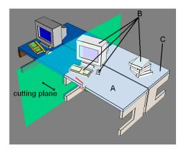
Figure 10. Group selection by directional dragging: The cutting plane is determined by the geometry of A and the dragging direction. Object A is selected and dragged into the direction. Objects B are selected since they are children of the existing group, and C is selected since it is a sibling of A and it is on the positive side of the cutting plane.
