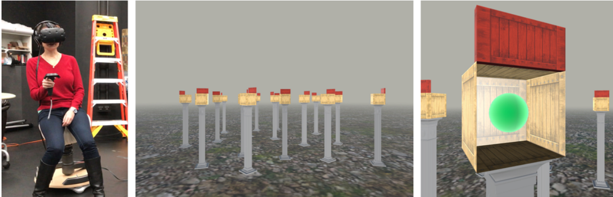
Figure 1: Left: Participant wearing an HMD (HTC VIVE) and sitting on the NaviChair locomotion interface. Middle: Visual stimuli of the virtual environment designed to eliminate all visual landmarks. Right: By approaching the box from its front side (the side denoted by a red banner), participants can make the box automatically open to see whether there is a ball inside, and collect the ball by touching it with the controller.
