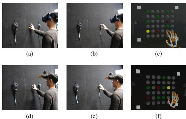
Figure 2: **Environments** and **Haptic feedback** conditions. First row shows VR (a) passive haptic feedback condition, (b) mid-air condition and (c) scene screenshot. Second row shows AR (d) passive haptic feedback condition, (e) mid-air condition and (f) scene screenshot. Since the Leap Motion covered the camera of the AR HMD, we could not capture a shot of the virtual scene in the AR condition.
