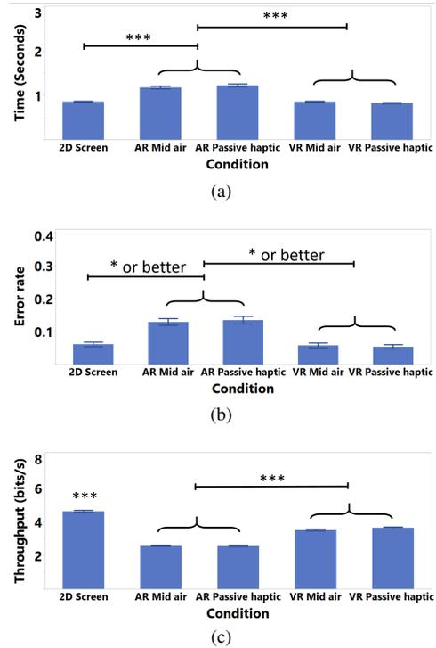
Figure 4: Analysis across all five experimental conditions for (a) time, (b) error rate, and (c) throughput.
