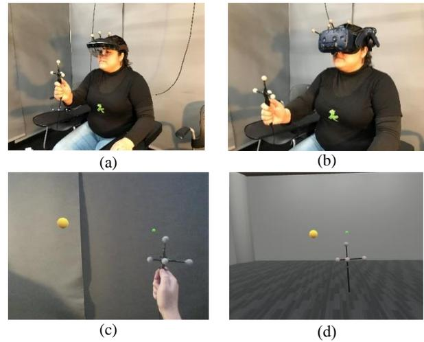
Figure 1 – Experimental setup with optical tracking markers. A user with the wand in the (a) AR headset and (b) VR headset. Participants' view for (c) AR and (d) VR.
