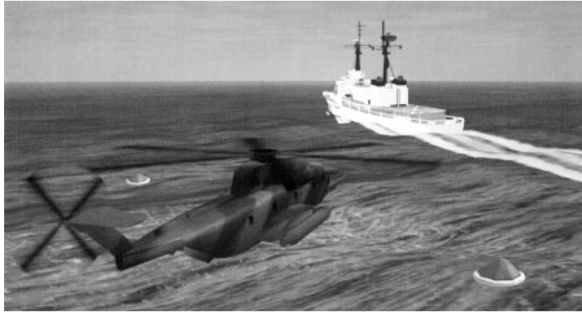
Fig. 1. Synthetic image demonstrating the degree of realism and sophistication available from current simulators. This example includes physics-based object and surface models, shading, focusing effects, motion blur, and atmospheric conditions. Although some effects are not modeled by this simulator, a perception system that performs badly on this kind of imagery can be expected to fail in a similar situation in reality (image source: Evans & Sutherland).
