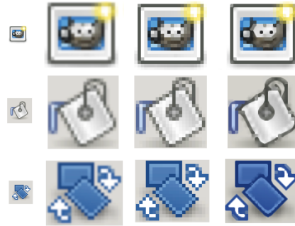
Fig. 5. Low-resolution icons (small, left column) scaled using naïve texture-scaling (second column), image up-scaling (third column) and HQx respectively (right).
