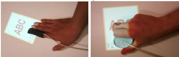
Figure 2: TNT-hand (left) and TNT-block (right) techniques [21] use embedded trackers to simultaneously translate and rotate digital objects.
