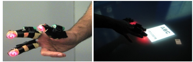
Figure 4: Fingerlings designed to add multi-touch capability (left), reaching to transform a 2D virtual object (right).
