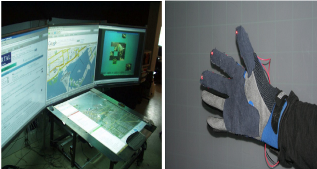
Figure 1. An overview of the apparatus: (a) MULTI system [9] consisting of 3 interactive walls and a table top, (b) Touch-glove prototype designed to add touch functionality to MULTI.
